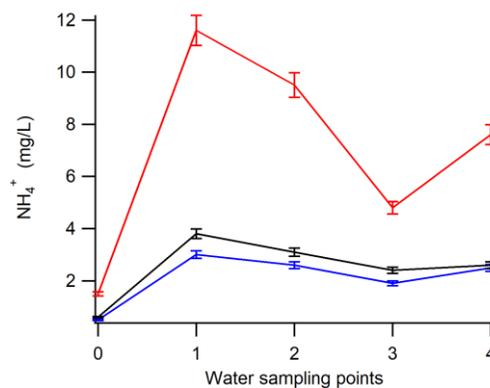
**Fig. 3** - Ammonium ion ( $NH_4^+$ ) concentration (mg/L) measured on water samples collected from Selva del Lamone reserve. Blue line, black line and red line refer to 14 July 2023, 31 July 2023 and 28 August 2023 water sampling campaigns, respectively. Surface water sampling points on X-axis: 0 (Mezzano lake), 1 (Valle Latera), 2 (S. Maria di Sala bridge), 3 (Salabrone waterfalls), 4 (Farnese water treatment plant). %RSD  $\leq$  5%.
