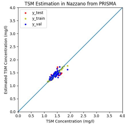
**Fig. 1** - Scatterplot of TSM concentration derived from Landsat 8 physical model vs. TSM estimated with AI model in Nazzano reserve.
